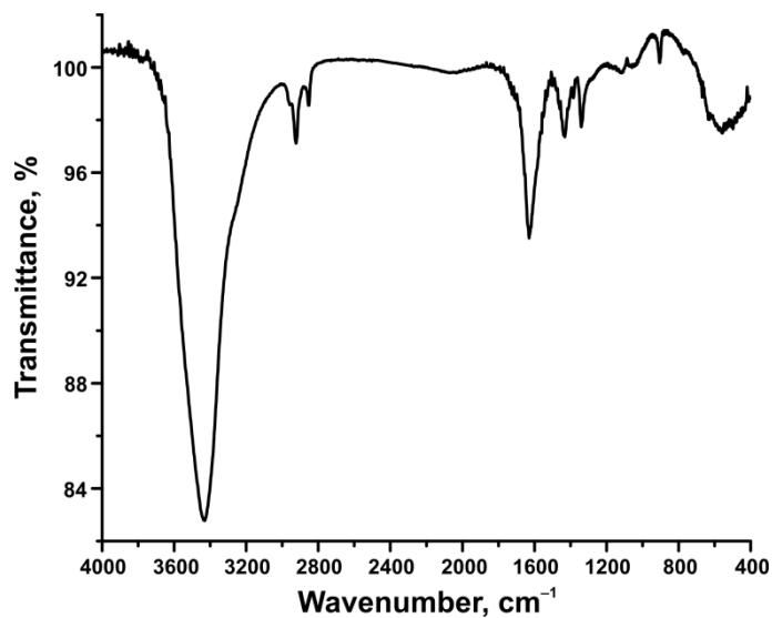
**Figure S2.** FTIR spectrum of  $\text{Na}_6\text{mell}\cdot 13\text{H}_2\text{O}$ .
