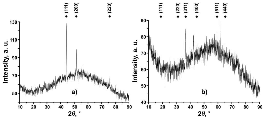
**Figure S3.** XRPD patterns of Co (a, ● Card No. 01-089-7093) and  $\text{Co}_3\text{O}_4$  (b, ♦ Card No. 01-078-1969).
