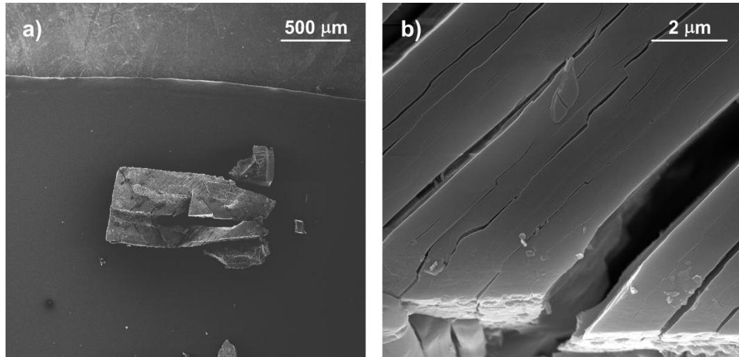
**Figure S1.** FESEM images of single crystal of **1** at magnification of 73 x (a) and layers of **1** at magnification of 20.0 kx (b).
