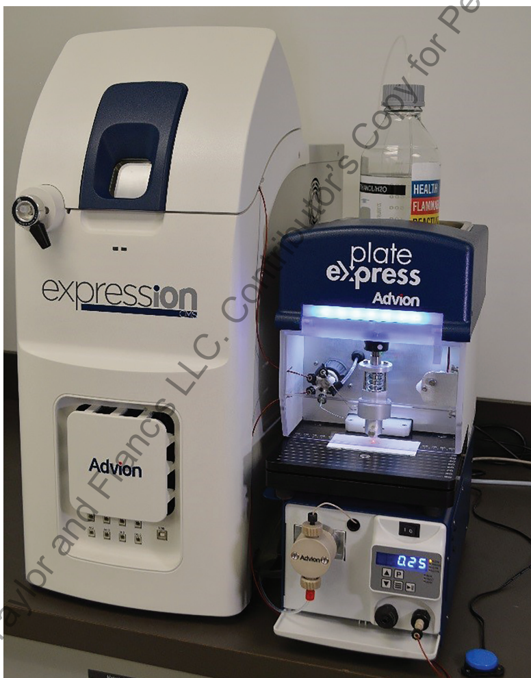
FIGURE 22.2 Advion Automated TLC-Compact Mass Spectrometry system. (From Jack Henion, Advion, Inc., Ithaca, New York. With permission.)
