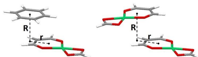
Figure 3. The geometrical parameters describing the benzene-chelate and chelate-chelate stacking interactions are the horizontal displacement (offset) r of the centers of interacting rings, and the normal distance R , presented here as the shortest distance between benzene ring center and the chelate plane ( Bz-Ch ) or between center of one chelate ring and the plane of the other chelate ring ( Ch-Ch )
