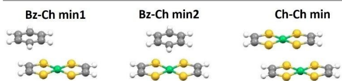
Figure 2. Minimum geometries of benzene-chelate ( Bz-Ch ) and chelate-chelate ( Ch-Ch ) stacking interactions of dithiolenic chelate rings of Ni. The corresponding potential energy curves are presented in ESI (Figures S4 and S6).
