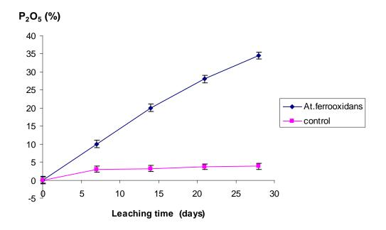
Figure 2 - Percentage phosphorus recovery (%  $P_2O_5$ ) from phosphate ore during leaching experiments
