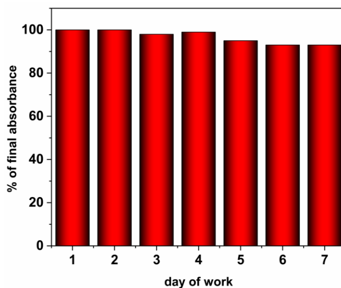
Figure 8. Changes in the final absorbance during seven days of work with the same electrode.
