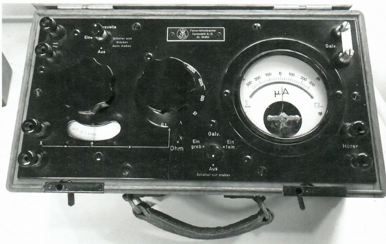
Whitstone bridge, Felten & Guillaume , Germany, 1930s. Museum of Science and Technology, T:6:202
