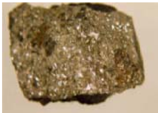
Slika 7.- Makro izled ferotitana Figure 7.- Macro view of ferrotitanium
