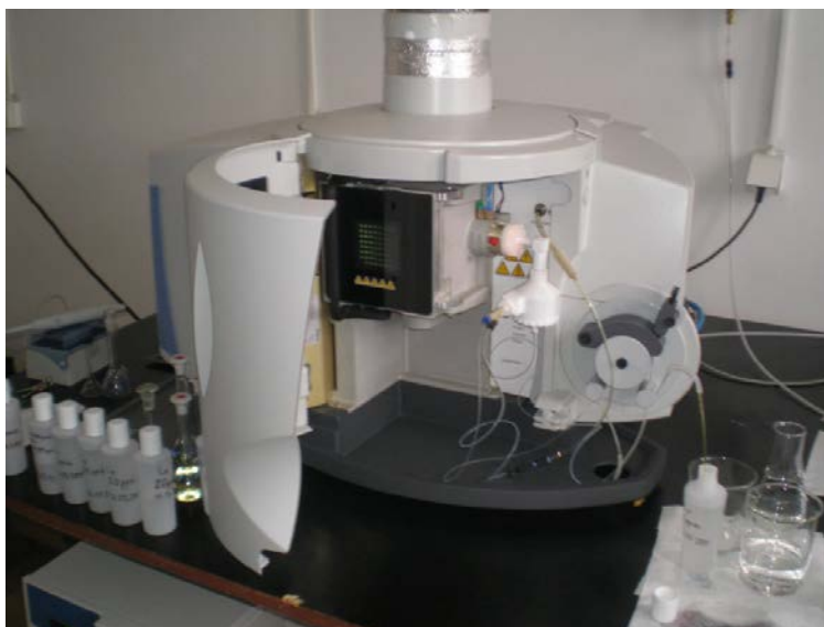
Slika 29. ICP-OES, Thermo Scientific iCAP 6500 Duo instrument, Thermo Fisher Scientific, Cambridge, UK.
