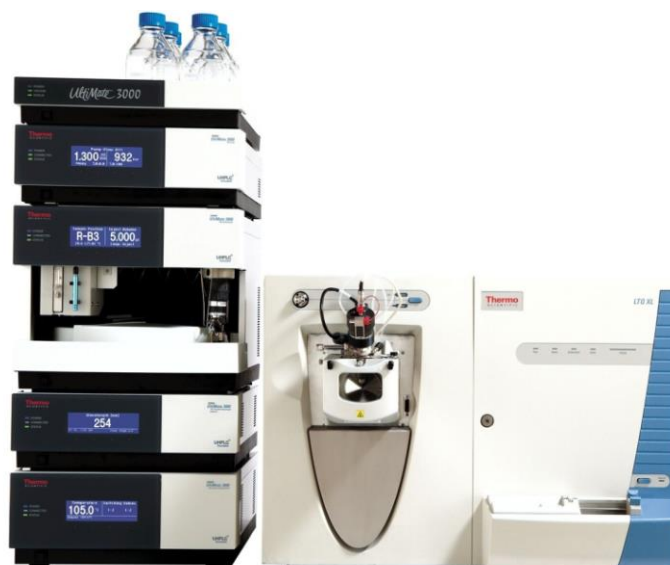
Slika 6. Ultimate 3000 HPLC-DAD-TSQ Quantum Access Max maseni spektrometar.
