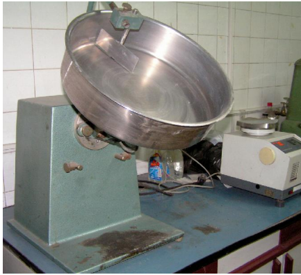
Figure 2. Laboratory Pelletization disc unit Eirich TR-04, diameter 0.4 m
